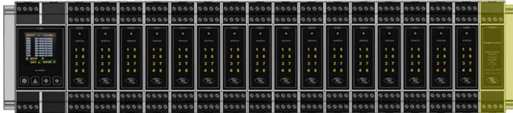
It is essential that the ICENI/PS-01 module is positioned to be the last module in the node.
