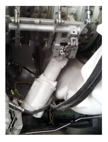
thus providing positive shut off of the compressor discharge air thus maintaining compressor performance.
