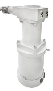
This is a position servo assembly consisting of a digital electronic controller, rotary servo motor and rotary to linear gearbox. In application, the unit is usually mounted in trunnions and connected by a spherical jointed coupling to a mechanism which transfers the linear motion to rotate several stages of variable inlet stator blades on an axial compressor.
