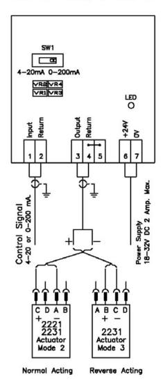
In order to comply with EMC requirements the converter must be fitted in a steel plate enclosure!
