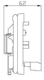
Mountig on Rail G32 or Hatrail 35 DIN EN 60715 The module is fitted with a self-resetting fuse. The LED will indicate power supply available (green) or fuse interrupted (red).
