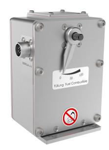
times can be gained. In case of voltage loss a return spring ensures setting back to zero position. Optionally the actuator is available without return spring. A contactless feedback system is integrated onto the governors output shaft offering an electrical position signal to any external control unit. A current limitation which is activated 20 seconds after the actuators might be blocked mechanically prevents them from damage by overheating.
