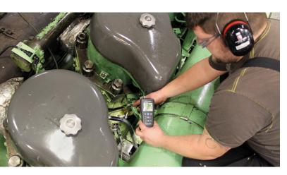
Vibration measurements show a smoother engine run after the conversion
