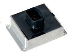
connection of an actuator is made up by a cable moulted with DC 10. Signal input and communication is done via a Tyco-type plug. DC 10 is designed and optimised to act in concert with high precision inductive feedback with PWM output. So it can serve as positioner control combined with appropriate actuators as well.
