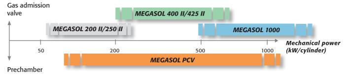
inlet valve Guideline only, MEGASOL size depends on gas quality and pressure difference between gas and boost pressure
