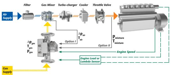
With additional information on the air or mixture mass flows the gas dosing system can be extended to a complete lambda control system (LC). In the standard version the flow is obtained by measuring the pressure difference over the calibrated Venturi gas mixer. A setpoint may be derived from engine load or from a lambda sensor.
