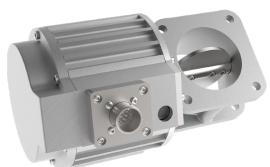
The actuator driving the valve is equipped with a multi-polar magnetised permanent magnet system mounted directly on the actuator shaft. This design allows generating powerful torque in both directions of working equally. Result of the direct acting gearless function are very fast response times.
