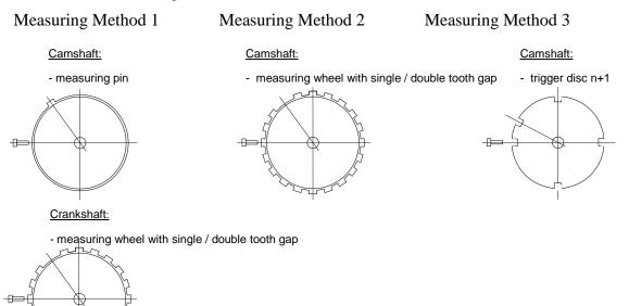
Figure 12: Pick-up configuration
