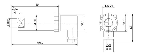
Figure 6: Boost pressure sensor with contact plug
