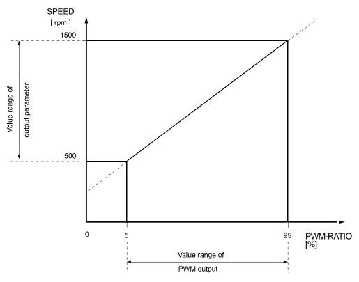
Figure 10: Reading out a parameter via a PWM output
