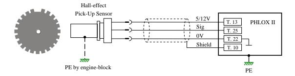
Connection to inductive shaft position sensor by ECU on the engine-block or other construction
