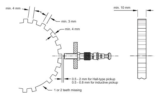
Figure 3: Distance of the speed pick-up
