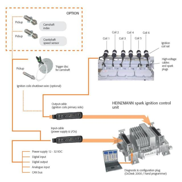
Figure 1: Example of configuration for 6-cylinder engine
