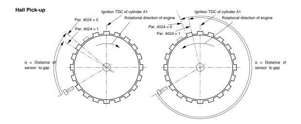
Figure 15: Crankshaft angle Hall pick-ups
