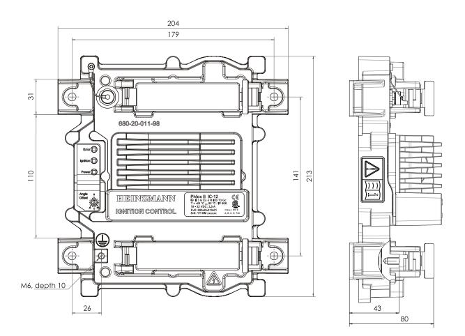
Figure 2: Dimensional drawing of PHLOX II control unit
