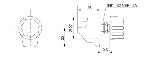
Figure 7: Potentiometer SW 02 - , 1- turn
