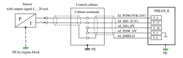
Connection to customer ECU inside control-cabinet and use of common power -supply.
