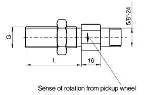
Figure 5: Hall sensors with contact plug
