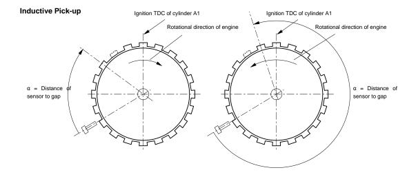
Figure 16: Crankshaft angle inductive pick-ups
