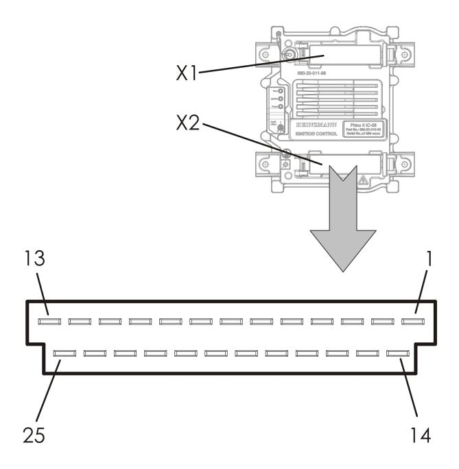
Figure 9: Connector X1 and X2
