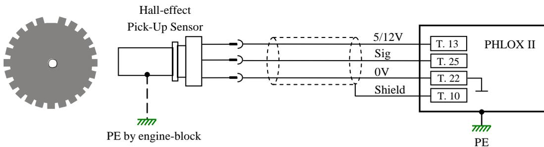
Connection to inductive shaft position sensor by ECU on the engine-block or other construction
