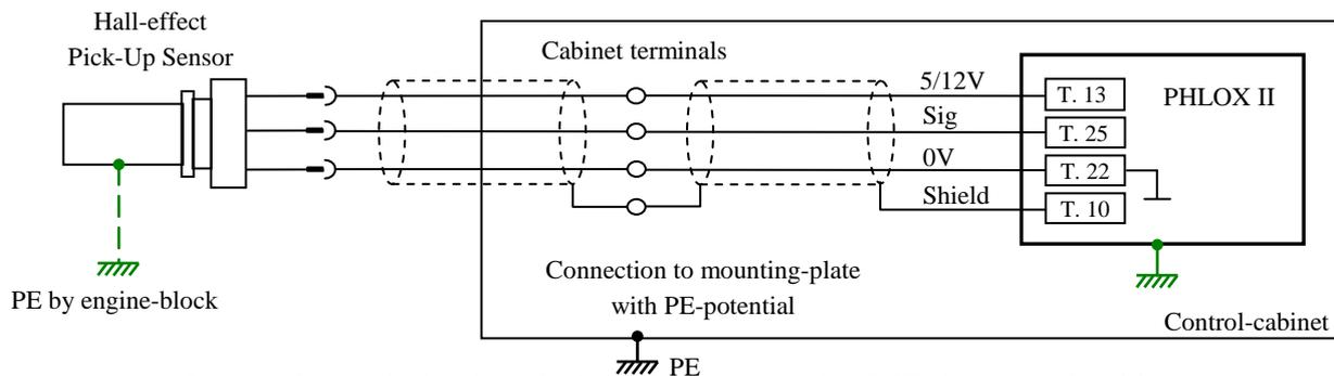
Connection to inductive shaft position sensor by ECU in control-cabinet
