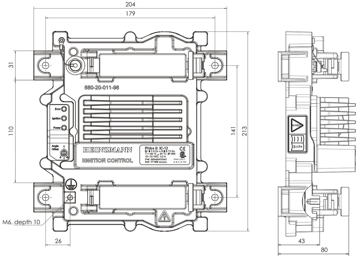
Figure 2: Dimensional drawing of PHLOX II control unit
