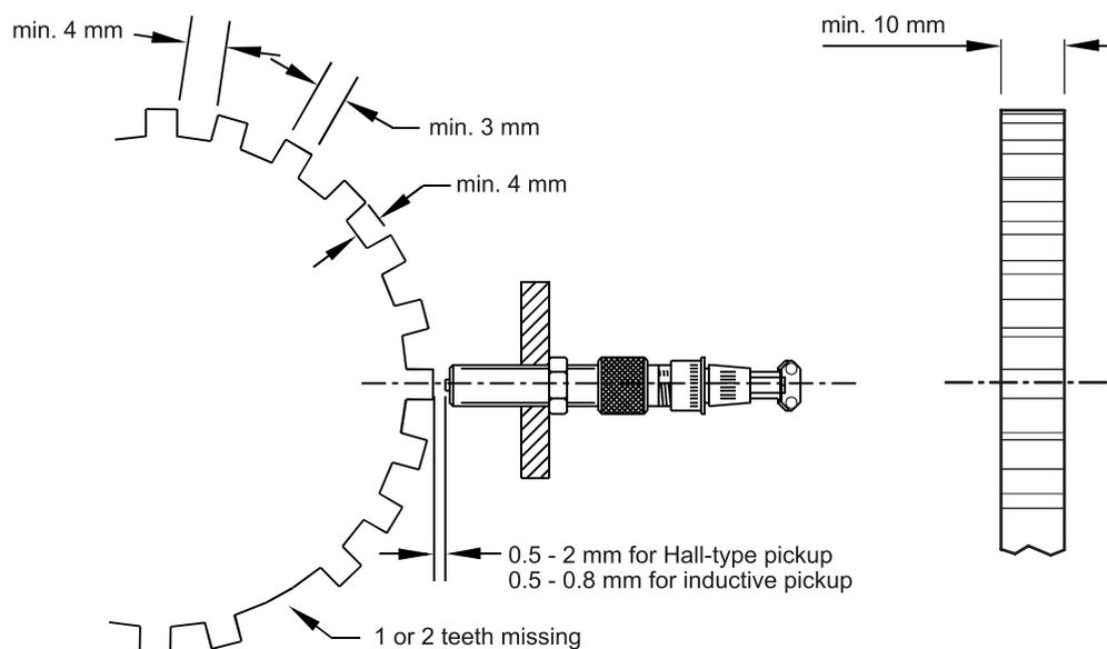
Figure 3: Distance of the speed pick-up
