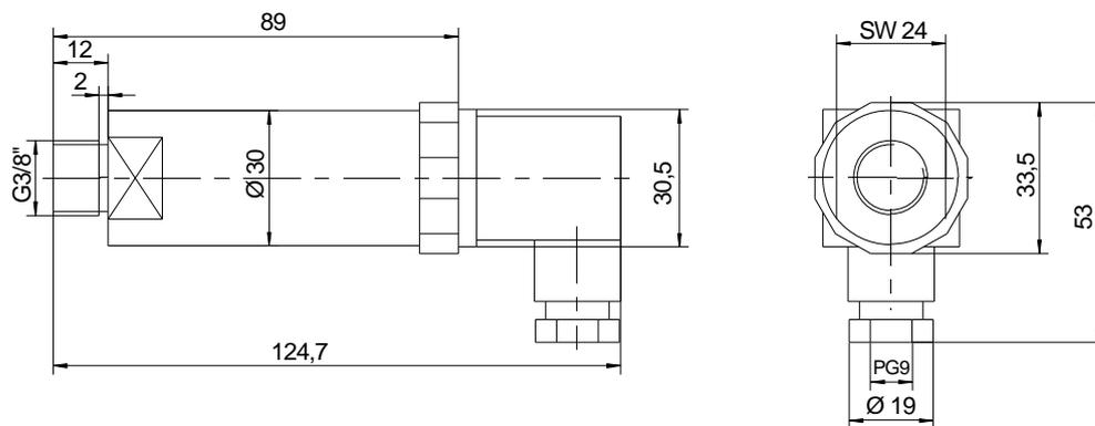
Figure 6: Boost pressure sensor with contact plug
