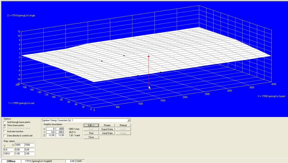
It is, of course, possible to set up a fix cylinder individual ignition angle correction, which is independent of speed or load. To do this, delete the second column and the second diagram and setup the correction value in the upper left cell, as in the following example:
