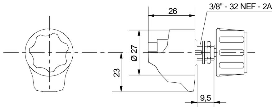
Figure 7: Potentiometer SW 02 - , 1- turn
