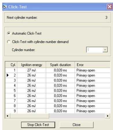
Ignition test on all cylinders alternatively
