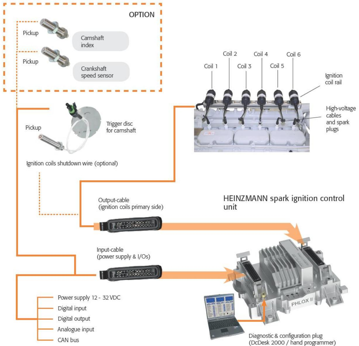
Figure 1: Example of configuration for 6-cylinder engine
