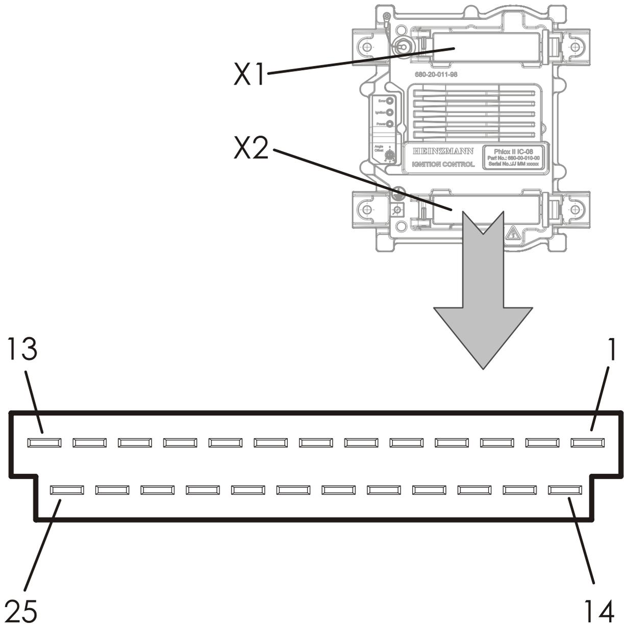
Figure 9: Connector X1 and X2
