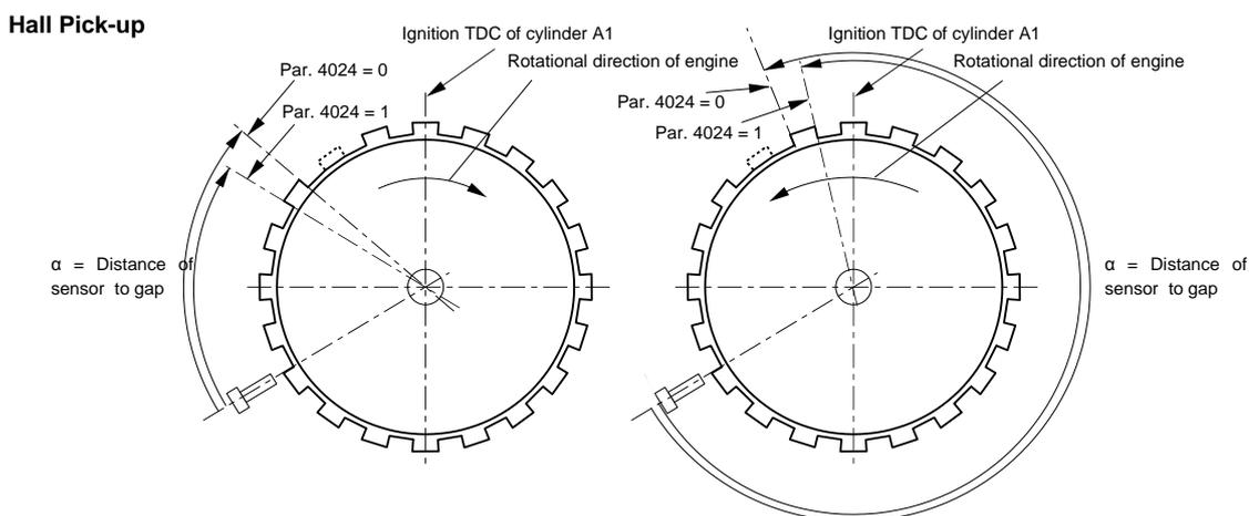
Figure 15: Crankshaft angle Hall pick-ups
