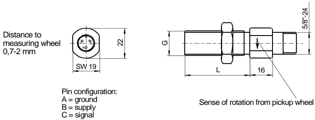
Figure 5: Hall sensors with contact plug
