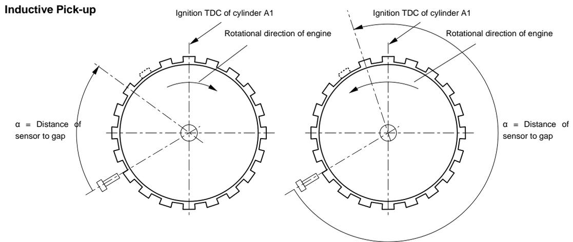
Figure 16: Crankshaft angle inductive pick-ups
