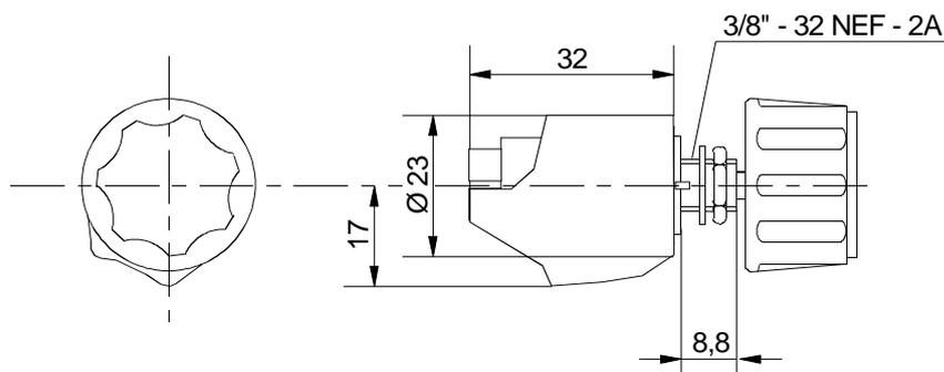
Figure 8: Potentiometer SW 02 - , 10-turn
