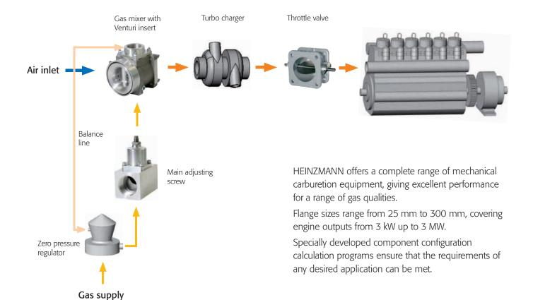
Provided that a zero pressure regulator is used, the Venturi principle ensures that the desired air fuel ratio remains stable over differing speed and load conditions.
