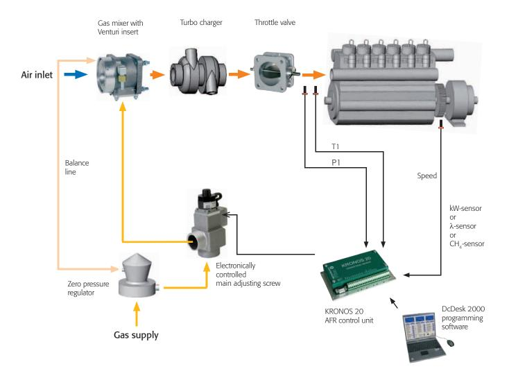
Based on the same Venturi principle as the KRONOS 10, the KRONOS 20 provides an electronically controlled main adjusting screw, a digital control system and all necessary sensors.
