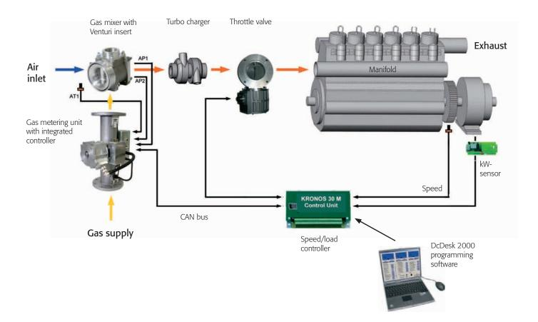
The KRONOS 30 M does not require a zero pressure regulator and includes a gas metering unit able to handle pressure changes up to a ratio of 2:1 and a pressure range 30 – 200 mbar. It is also tolerant to wet biogas and other corrosive contaminants.
