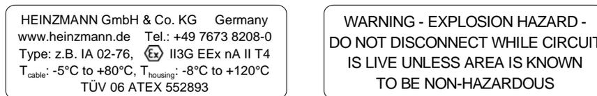
Figure 8: Signboard at Magnetic Pickup Cable, Front and Back Sides
