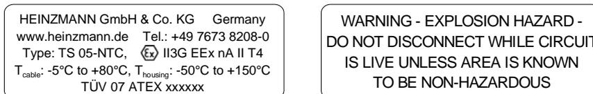
**Figure 12: Signboard at Temperature Sensor Cable, Front and Back Sides**
