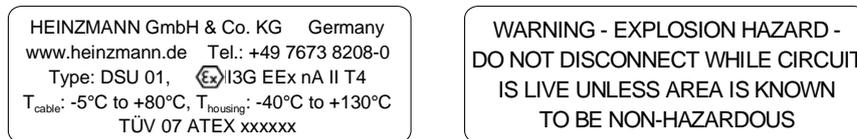
Figure 10: Signboard at DSU Sensor Cable, Front and Back Sides
