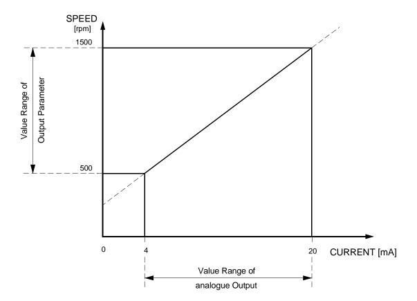
Figure 25: Reading out a Parameter via an analogue Output
