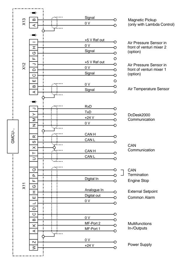
Figure 22: Wiring Diagram ELEKTRA
