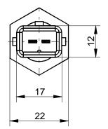
Figure 11: Measurements of Temperature Sensor TS 05-NTC
