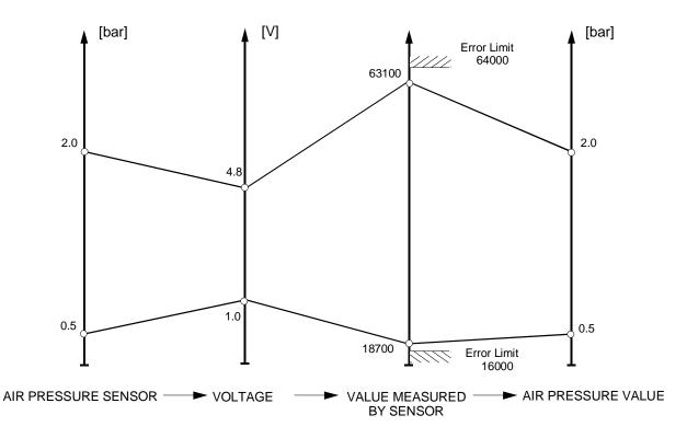
**Figure 24: Calibration Procedure**
