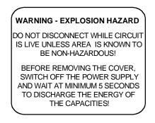
Figure 21: Label 3 with warnings about removing the plugs and the cover
