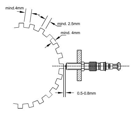
Figure 6: Clearance of Pickup
