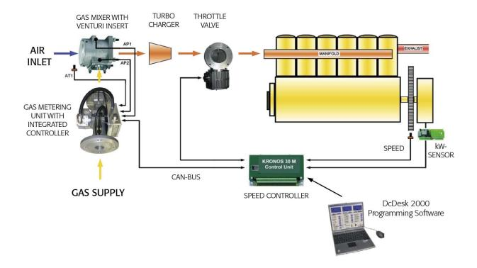
Figure 5: Lambda Control System with Speed / Load Control System (KRONOS 30-M)
