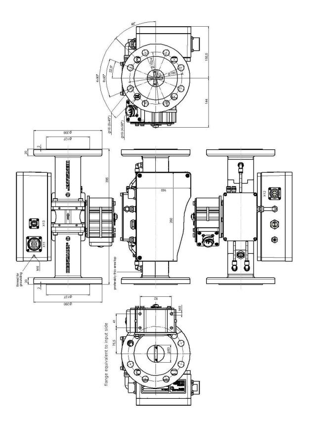
Figure 16: Dimensioned drawing of GMCU-50-LC
