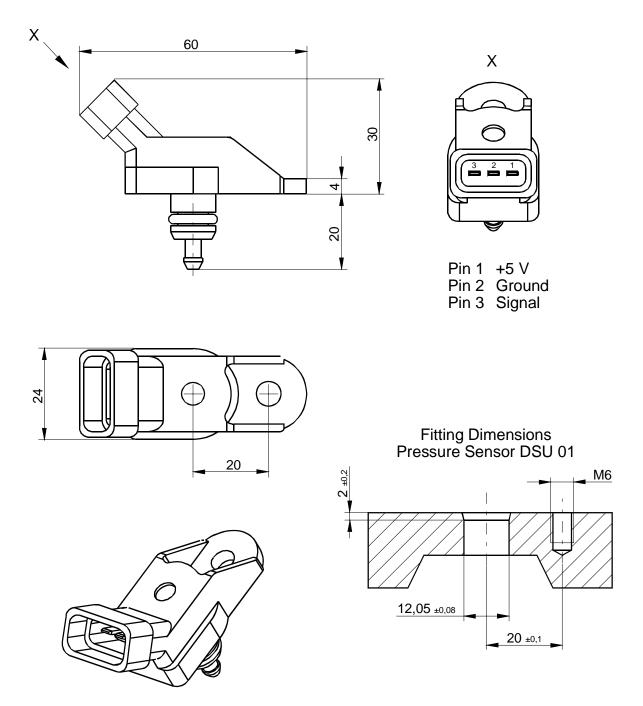
Figure 9: Measures of Pressure Sensor DSU 01
