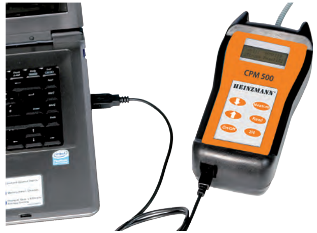
CPM 500 connected via USB cable to PC
