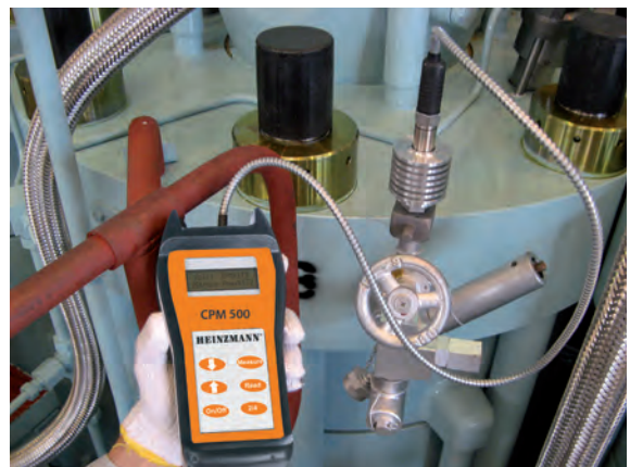
CPM 500 with HTT sensor mounted in adapter at the indicator valve
