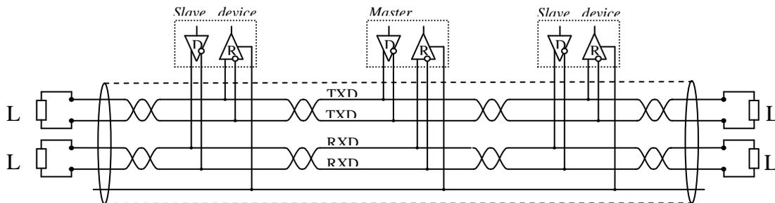
In order to obtain optimum transmission quality and/or signal quality, particularly over long distances, the data line is to have a termination as a twisted data conductor pair at both extremities according to **Figure 9**. For this, termination load must correspond to the characteristic impedance of the data line.
