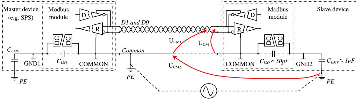
$U_{CM1}$  – Common mode voltage from transmitter with interference induced among the conductors within the bus cable.
