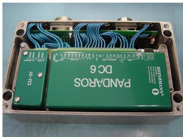
**Fig. 28: TWIN-PANDAROS, printed circuit board with position of the terminating resistors (photo)**
