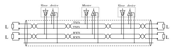
In order to obtain optimum transmission quality and/or signal quality, particularly over long distances, the data line is to have a termination as a twisted data conductor pair at both extremities according to **Figure 9**. For this, termination load must correspond to the characteristic impedance of the data line.
