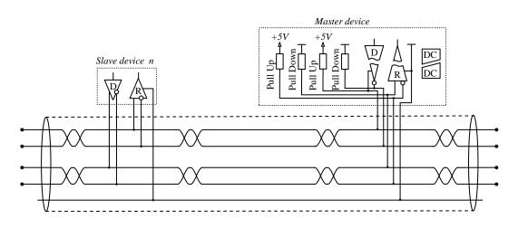
Figure 10: Line polarization in a four-wire-system
