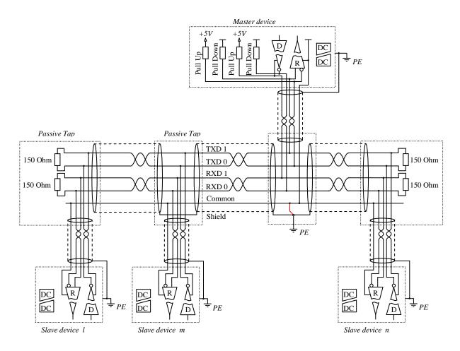
Figure 5: Signal definition – four-wire-system
