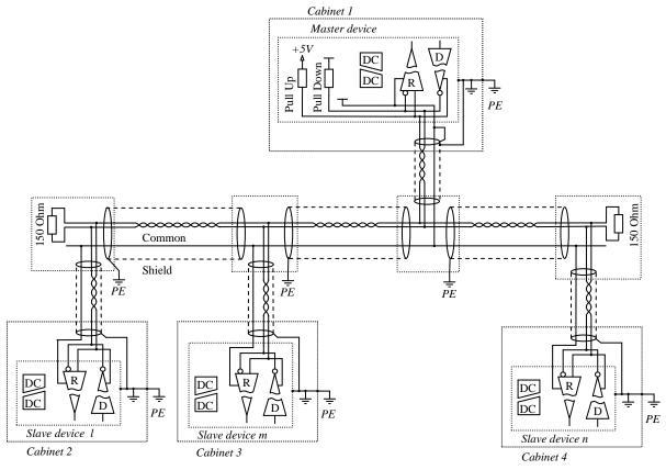
Figure 7: Reference potential and shield
