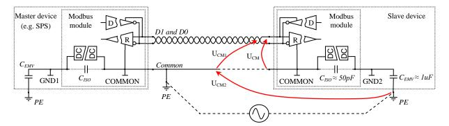
$U_{CMI}$  – Common mode voltage from transmitter with interference induced among the conductors within the bus cable.  $U_{CM2}$  – Interference induced between Common line and protective earthing conductor.
