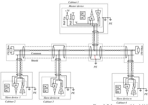
Figure 8: Reference potential and shield
