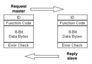
Figure 1: Request-reply-cycle
