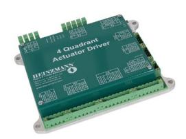
The 4Q actuator driver comes equipped with analogue, digital and PWM inputs as well as analogue and digital outputs. All inputs are isolated. The driver is short-circuit-proof and protected against polarity reversal.
