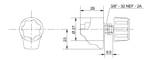
Figure 8: Potentiometer SW 01 - 1 - b
