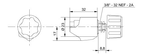
Figure 9: Potentiometer SW 02 - 10 - b
