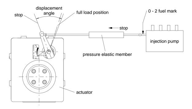
Figure 13: Linkage for Diesel Engines
