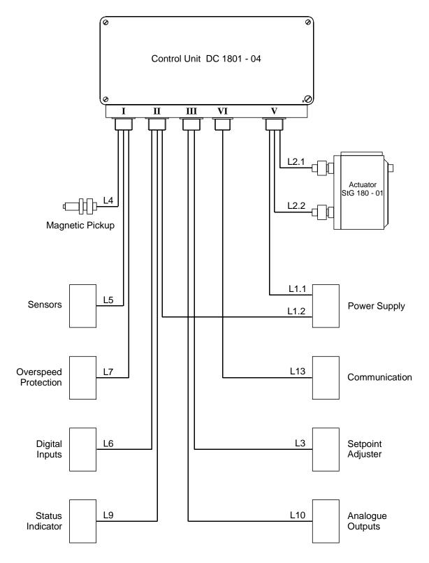
Figure 20: Harness with Cable Numbers
