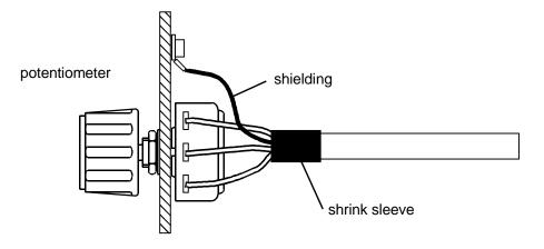
Figure 16: Shield Connection without Plug
