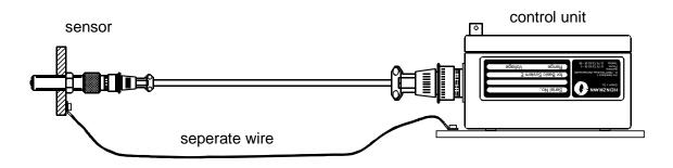
**Figure 15: Connection of seperat Wire**
