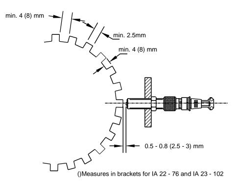
Figure 2: Clerance of Pickup
