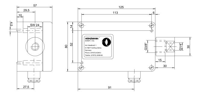
Figure 7: Boost Pressure Sensor with Housing
