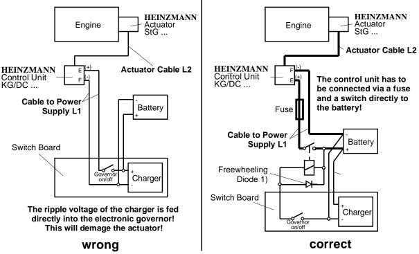
1) Coils (e.g. stopping solenoid, gas valve) have to be equipped with a protective circuit to eliminate high indunctance votages. Diode type e.g. 1N4002
