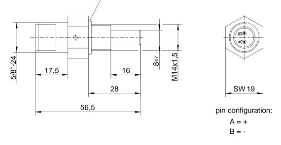
Figure 4: Temperature Sensor TS 01 - 28 - PT 1000
