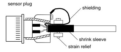
Figure 17: Shield Connection in the Plug
