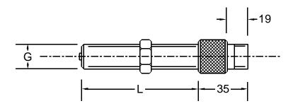
Figure 3: Magnetic Pickup
