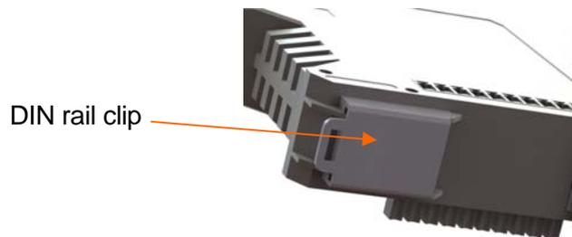
An IcenI node can be mounted in both vertical and horizontal orientations according to terminal rail layout. Assembly of the IcenI node can be achieved in one of two ways:
