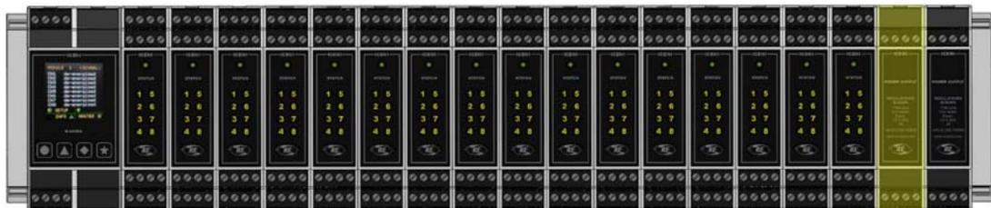
Where the node contains more than one IcenI redundant power supply, the redundant power supplies should be fitted to the left of the IcenI main power supply module, but after all IcenI signal conditioning modules.
