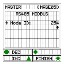
Using the 'dec' or 'inc' pushbuttons, the character numerical value can be nudged down or up one increment where the increment is equal to the character position. i.e. if the selection cursor is in the 'tens' column then when 'inc' pushbutton is pressed, the value will be increased by 10.
