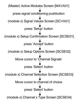
The screen will present the various signal type options for the specific signal channel to be configured. (Edit is by selection from a list.)
