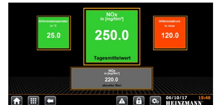
Measured value display in 7" TFT display
