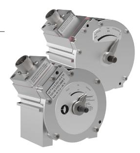
of powerful torque in both directions of working equally. Very fast response times are the result of this direct acting and gearles function. Optionally a return spring can be mounted on the output shaft to ensure setting to a zero position in case of voltage loss or similar.
