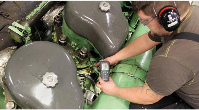
Vibration measurements show a smoother engine run after the conversion
