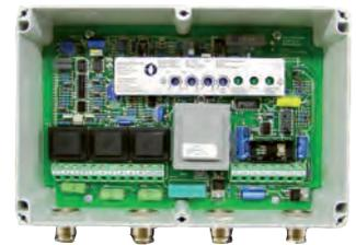
This synchroniser unit incorporates a three-phase comparison of voltage, frequency and phase angle (indicated by LEDs) between the bus bar and the generator and controls the generator speed.
