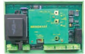
Accessory for existing LMG 11 load share units to ramp up or down the load of generators, connected to the grid. Also usable as a speed ramp unit for analogue speed governors.
