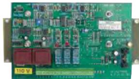
The voltage matching unit will match the voltages between the generator and a bus. The output is a raise/lower signal which will interface to the AVR motor potentiometer.
