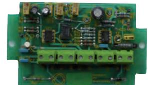
Accessory for load sensing, based on an actual load signal of 0 ... 5 V.
