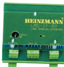
The Load Share Interface Unit LMG-IF-02 is used to couple load share lines of control systems, operating at different voltage levels.
