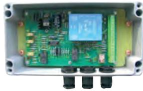
The unit allows soft load transfer from mains to generator, generator to mains and groups of generators to and from the mains.
