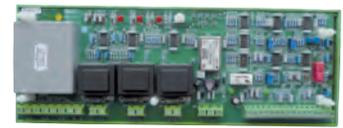
The KW-LKG-01 controller is designed for controlling multiple generators in parallel to a mains incomer.
