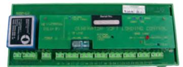
Accessories for LMG 11. The GSLU 01 unit allows parallel engines to isochronously load ramp in mains parallel and island applications.
