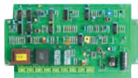
The power factor controller allows the control of reactive load via a motor potentiometer connected to the generator AVR.
