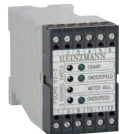
This unit has three output channels for cranking termination, under speed and over speed with a separate current or voltage output for a meter display.
