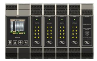
The master station can access the input process image to determine the plant status and also write to the output process image area to control plant devices. The network node is controlled by a master module that always occupies the first slot. A combination of input and output modules to suit the field requirements are then plugged into the right hand side of the master module to form the ICENI bus. The node is completed with a power supply module.
