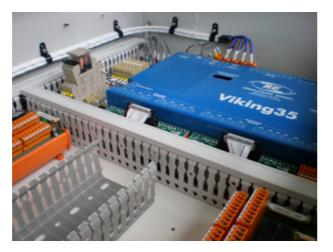
The engine protection provided by Viking Traction solutions provides de-rating with respect to measured parameters; this helps to ensure that the locomotive can continue to operate safely even if a fault is detected.
