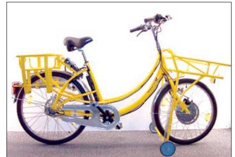
Fig. 1: Postal e-bike, equipped with HEINZMANN electric drive and control
