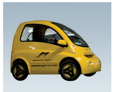
Fig. 3: Electrically driven „Kenguru“ vehicle for handicapped people, equipped with PERM motors
