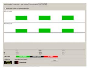
Figure 17: Window to monitore load sharing
