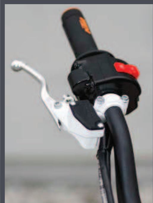
Twist and go... the current Freeride has both front and rear brakes controlled via levers on the bars.
