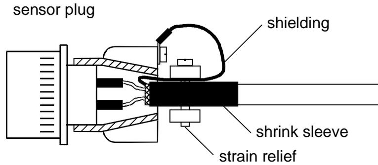
**figure 11: shield connection in the plug**
