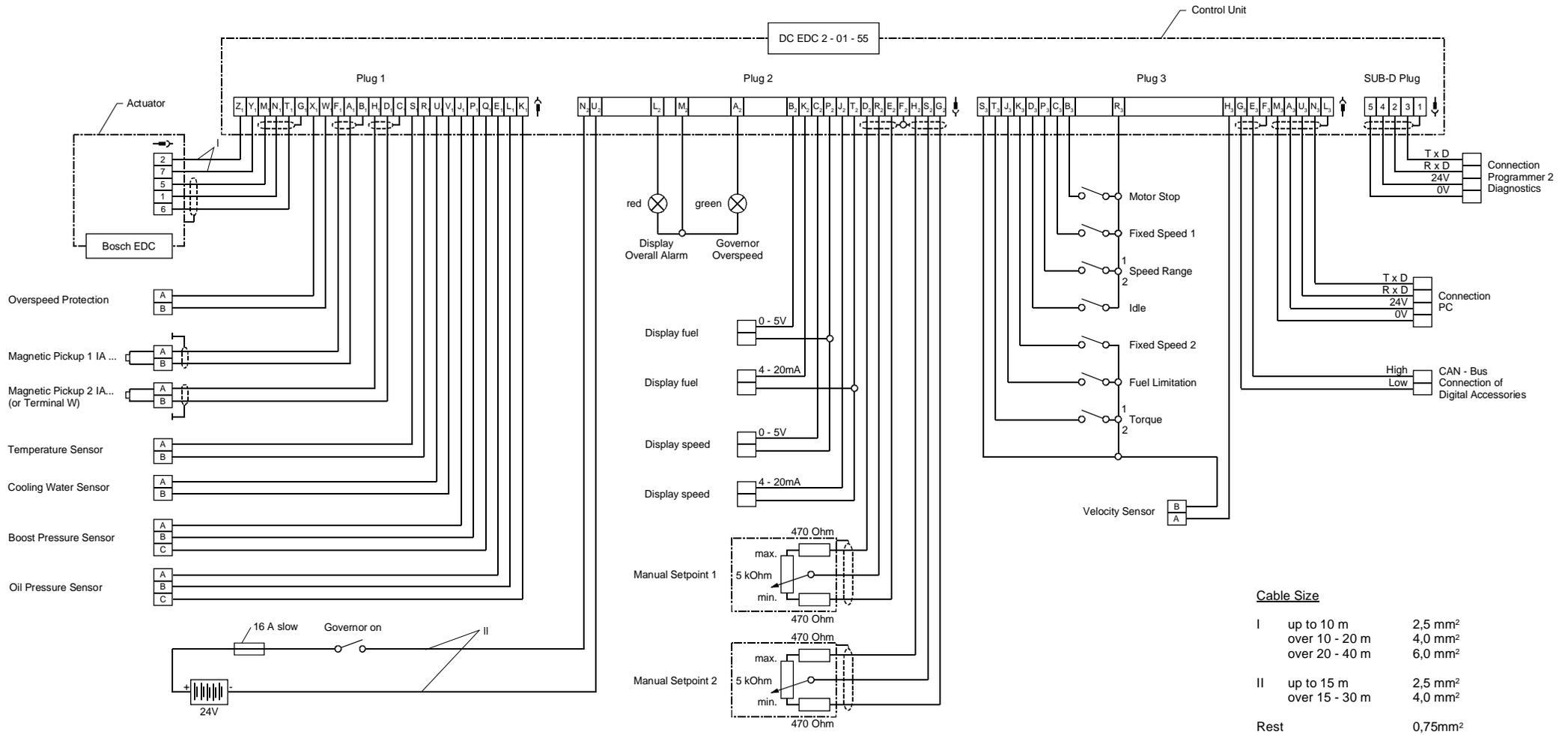
figure 16: connections with plugs (IP 55) for vehicle operation
