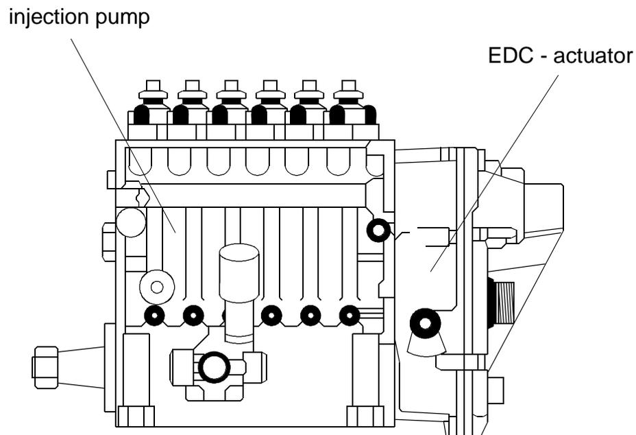
figure 8: sectional drawing of actuator
