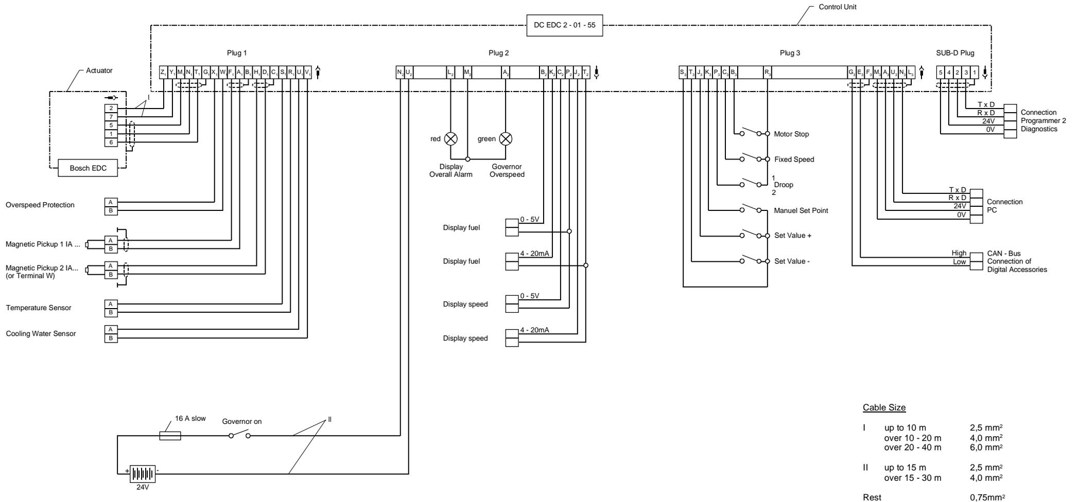
**figure 12: connections with plugs (IP 55) for genset with digital accessories**
