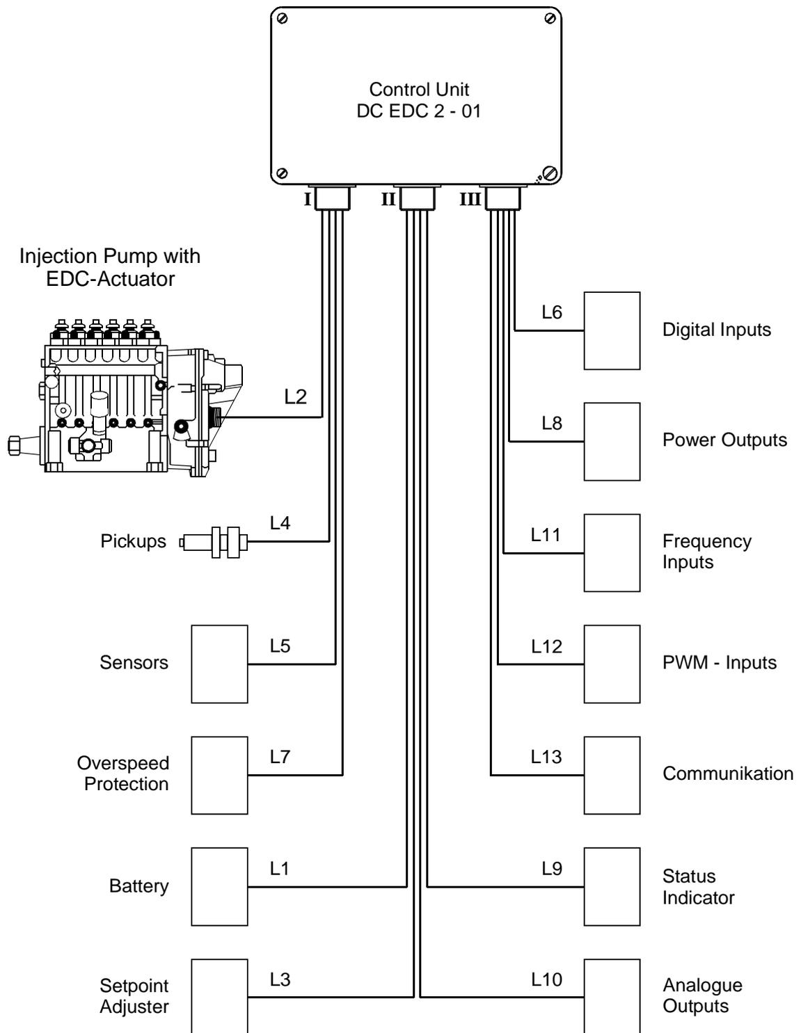
figure 27: harness with cable numbers
