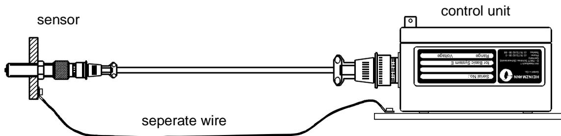
figure 9: connection of seperat wire
