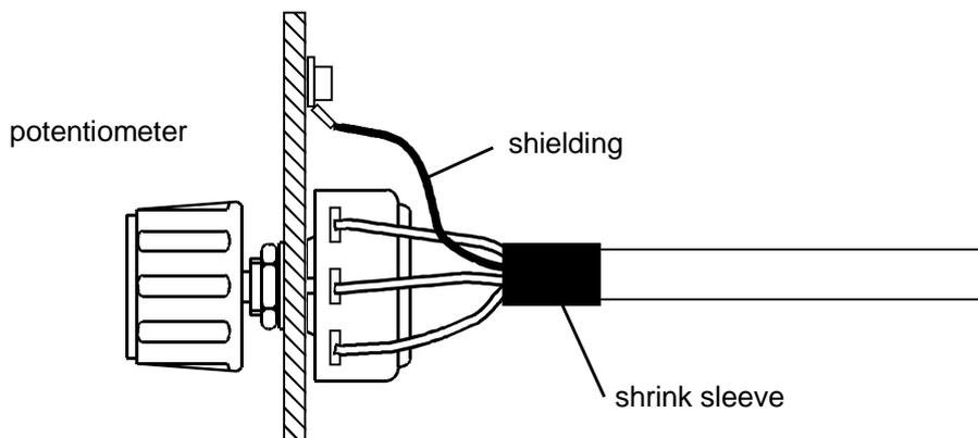
figure 10: shield connection without plug
