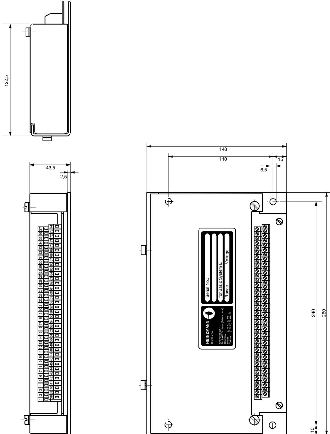
figure 7: housing of DC EDC 2 - 01 - 00
