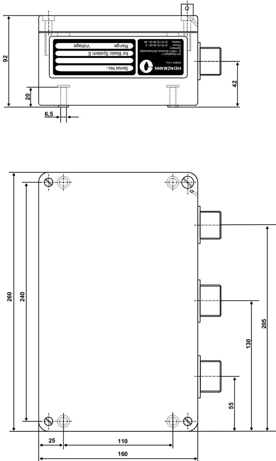
figure 6: housing of DC EDC 2 - 01 - 55
