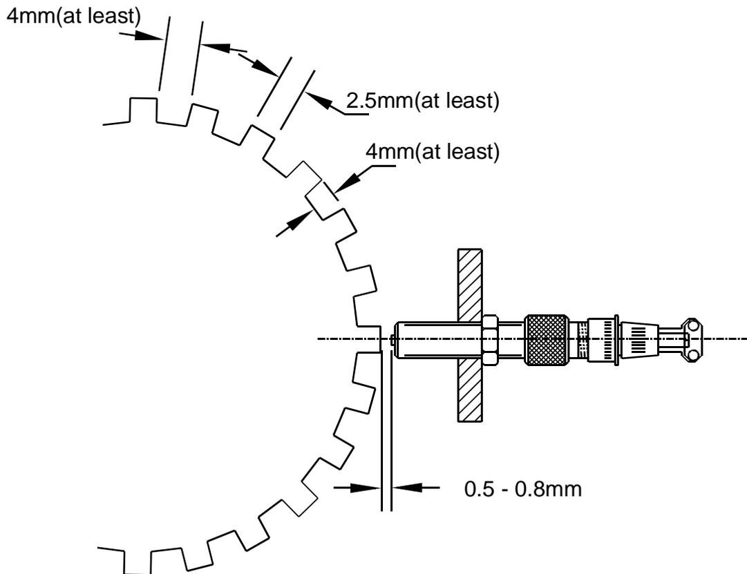
figure 2: clearance of pickup
